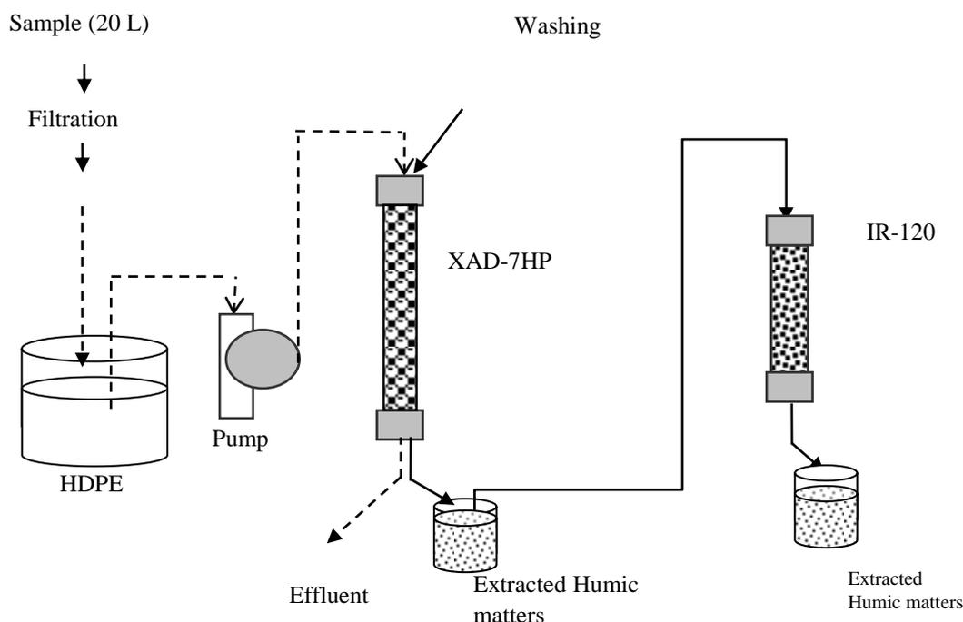
**Figure 1:** Schematic design of humic materials extraction
