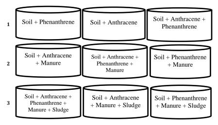
**Figure 1:** Pilotsstudy: 1. Control reactors; 2. Pilot containers containing chicken manure; 3. Pilot containers containing chicken manure + activated sludge
