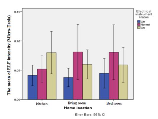
Figure 2: The mean intensity of ELF-EMF waves
