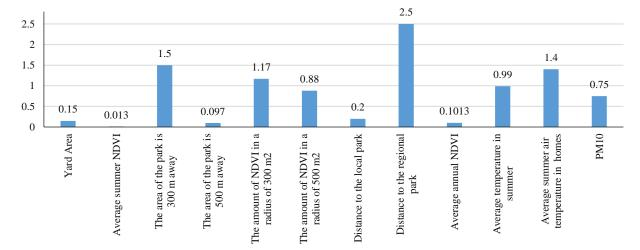
Figure 8: Investigating the effects of different variables on electricity usage using a neural network model
