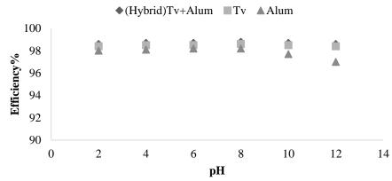
**Figure 6.** The impact of pH on the removal of turbidity (Tv:Thymus vulgaris, turbidity: 700 NTU, coagulant dose: 400 mg/L)
