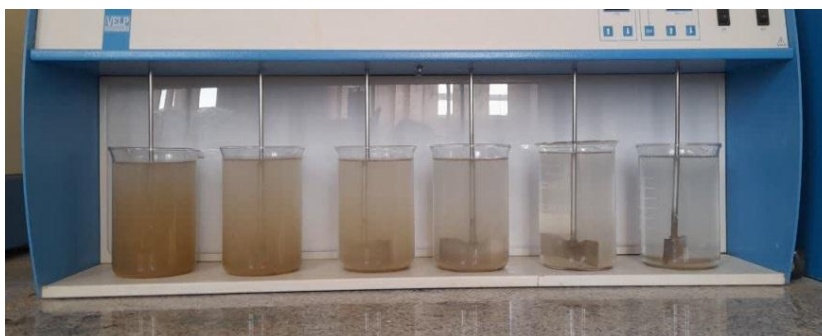
Figure 5-1. The impact of hybrid coagulant dose on removing turbidity (turbidity: 700 NTU, pH = 7).
