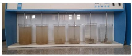
Figure 5-1. The impact of hybrid coagulant dose on removing turbidity (turbidity: 700 NTU, pH = 7).
