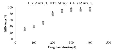
**Figure 5:** The impact of hybrid coagulant dose on removing turbidity (turbidity: 700NTU, pH = 7). **Tv:**Thymus vulgaris - **Tk:**Thymus kotschyanus - **Te:**Thymus eriocalyx.-Alum=Aluminium Sulfate- Al2(SO4)3)
