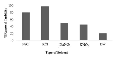
**Figure 8:** Influence of type of salt utilized for coagulant extraction on turbidity elimination (turbidity: 700 NTU, pH 7, salt concentration: 1 M, Tv dose: 400 mg/L).
