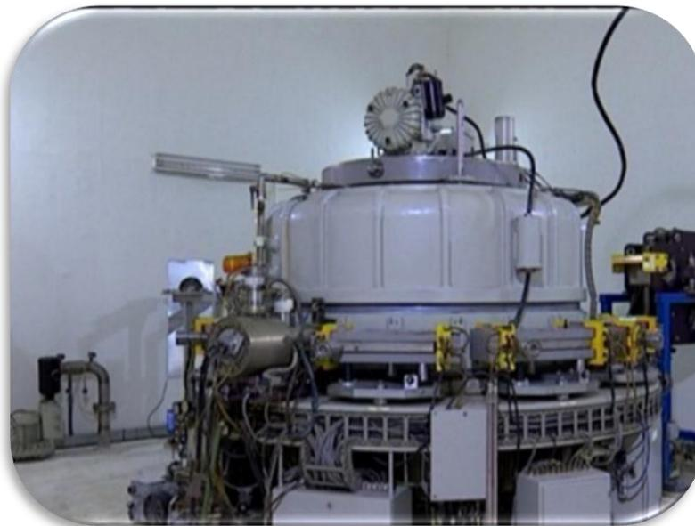
Figure 1: Rhodotron accelerator
