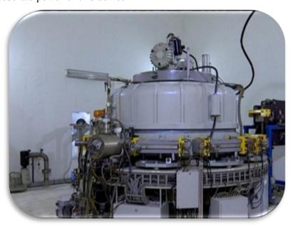
Figure 1: Rhodotron accelerator
