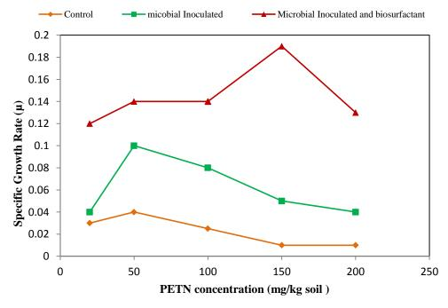
Figure 3: Specific microbial growth rate (µ) for 20, 50, 100, 150, and 200 mg/kg PETN in aerobic soil
