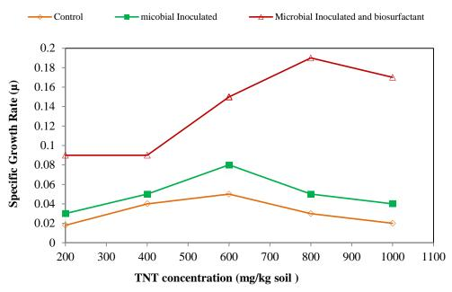
Figure 2: Specific microbial growth rate (µ) for 200, 400, 600, 800, and 1000 mg/kg of TNT in aerobic soil
