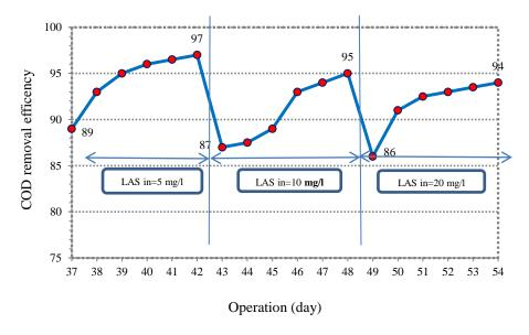
Figure 3: COD removal efficency during LAS adding through the operation time
