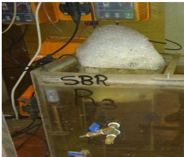
Figure 1: The SBR pilot with injection pump
