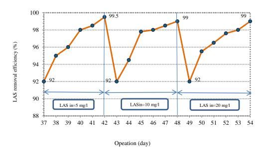
Figure 5: LAS removal efficiency in effluent during the operation time
