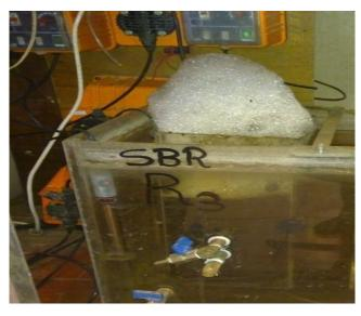
Figure 1: The SBR pilot with injection pump
