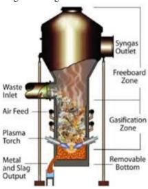
Figure 5: Plasma incineration process and source performance: Westinghouse Plasma Corporation<sup>34</sup>
