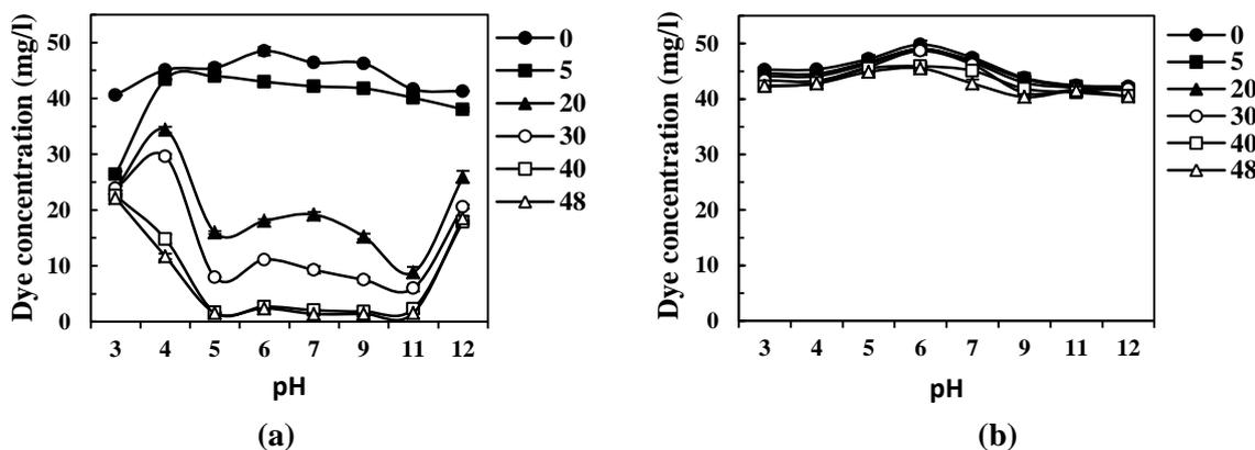
**Figure 4:** Effect of different initial pH values on dye removal from  $YS^{+C,50ppm}$  medium, (a) inoculated with *K. quasipneumoniae* GT7 and (b) non-inoculated (control) experiments during static incubation at 30°C
