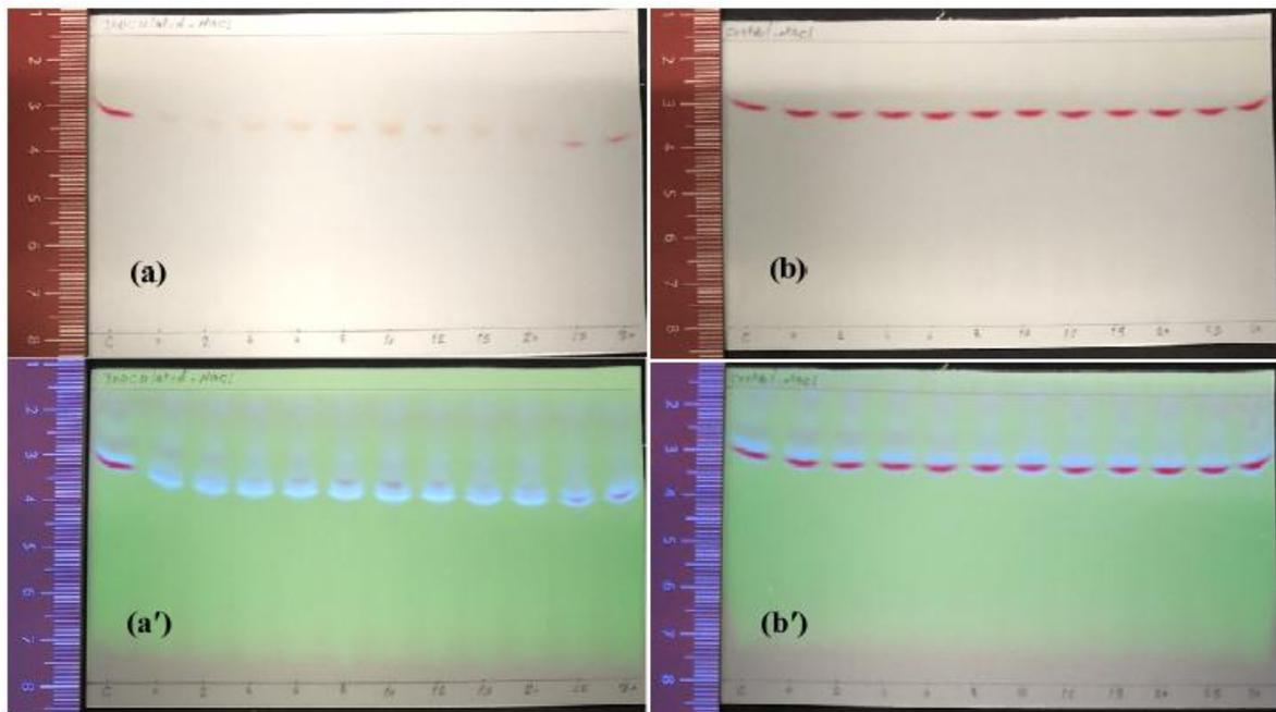
**Figure A1:** Display of TLC sheet samples extracted from YS<sup>+C,50ppm</sup> medium under various NaCl concentrations (0, 2%, 4%, 6%, 8%, 10%, 12%, 15%, 20%, 25% and 30%), (a & a') inoculated with *K. quasipneumoniae* GT7 and (b & b') not inoculated (control experiments) and statically incubated at 30°C for 48 h. Sheets were visualized under visible (a & b) and UV (a' & b') lights. The letter "C" on sheets stands for extract from YS<sup>+C,50ppm</sup> medium at the time of zero.
