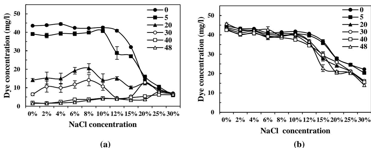
**Figure 2:** Effect of various NaCl concentrations on dye removal from  $YS^{+C,50ppm}$  medium, (a) inoculated with *K. quasipneumoniae* GT7 and (b) non-inoculated (control) experiments during static incubation at 30°C
