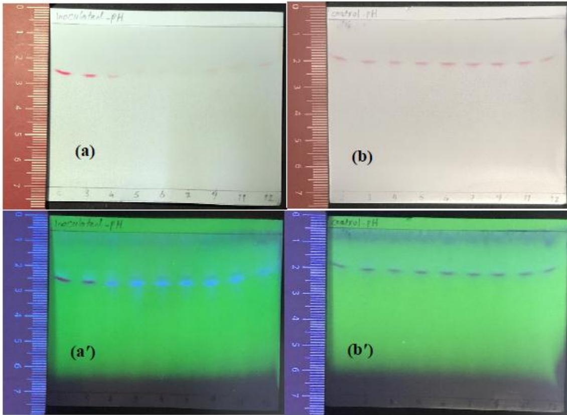
**Figure A4:** Display of TLC sheet samples extracted from  $YS^{+C,50ppm}$  medium with pH adjusted to different values (3, 4, 5, 6, 7, 9, 11, and 12), (a & a') inoculated with *K. quasipneumoniae* GT7 and (b & b') not inoculated (control experiments) and statically incubated at 30°C for 48 h. Sheets were visualized under visible (a & b) and UV (a' & b') lights. The letter "C" on sheets stands for extract from  $YS^{+C,50ppm}$  medium at the time of zero.
