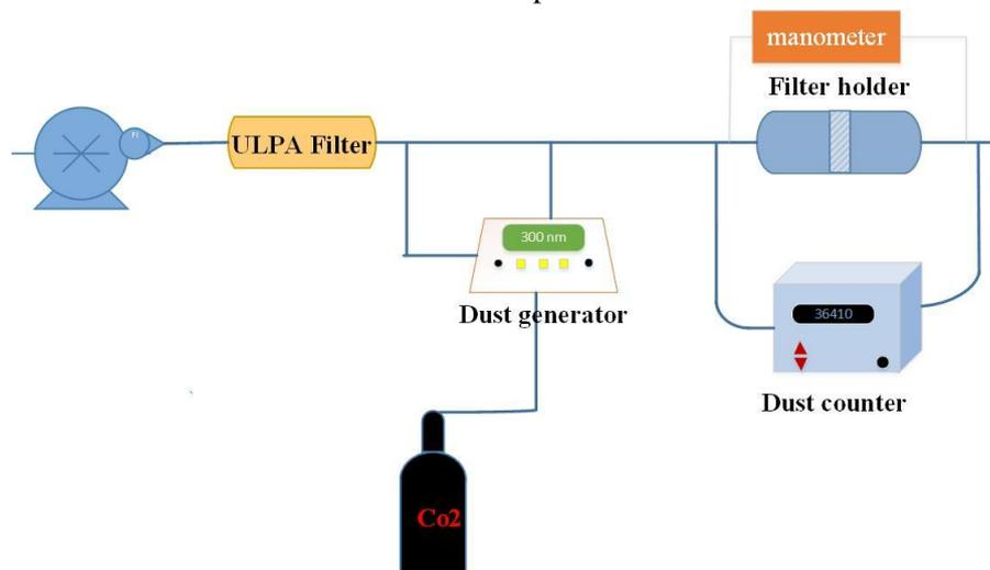
Figure 3: Measurement of filtration parameters in fabricated nanofibers
