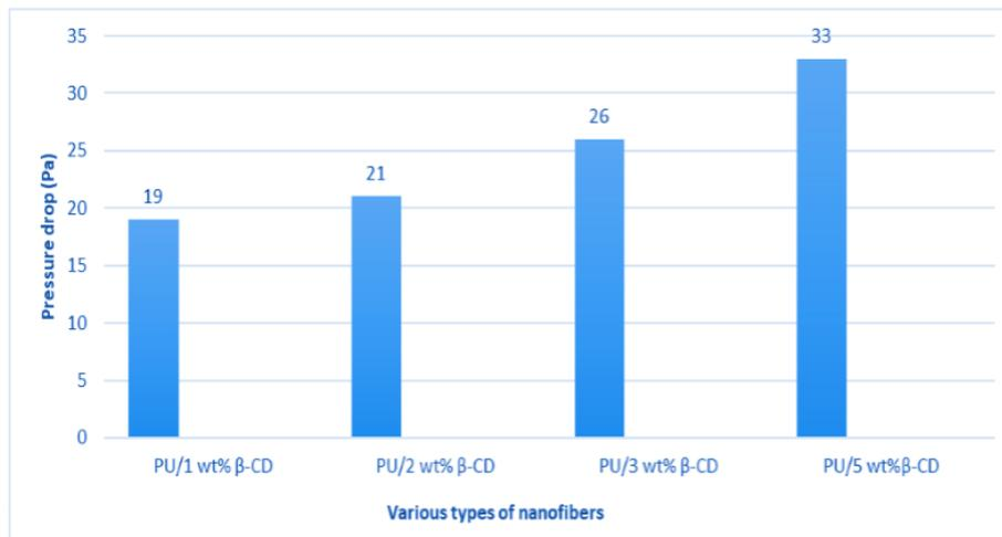
**Figure 8:** Pressure drop in composite nanofiber membranes
