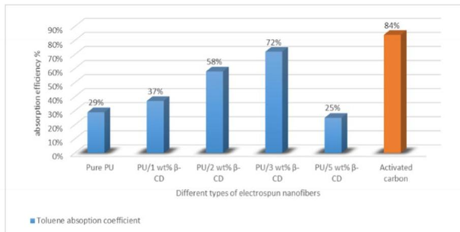
**Figure 10:** Toluene adsorption capacity of electrospun nanofibers and AC
