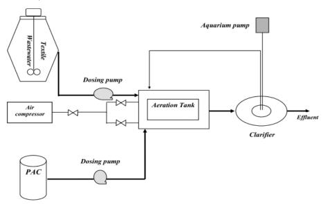
Figure 1: The schematic of the applied pilot
