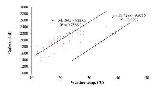
Figure 5: The volume of disinfected water vs. air temperature
