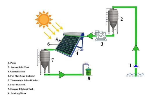
Figure 2: Schematic of the pilot
