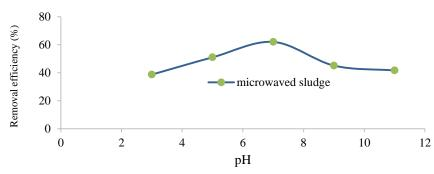
Figure 3: Effect of pH on the removal of 2,4 DNP on adsorbent microwaved sludge (experimental condition; adsorbent dosage =  $0.5 \text{ g} 40 \text{ mL}^{-1}$ ,  $C_0 = 50 \text{ mg L}^{-1}$  and contact time = 60 min)
