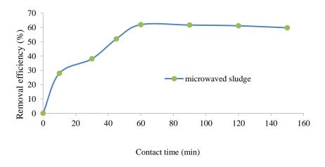
Figure 2: Effect of contact times on the removal of 2, 4 DNP by adsorbent microwaved sludge (experimental condition; adsorbent dosage =  $0.5 \text{ g } 40 \text{ mL}^{-1}$ ,  $C_0 = 50 \text{ mg L}^{-1}$  and initial pH = 7
