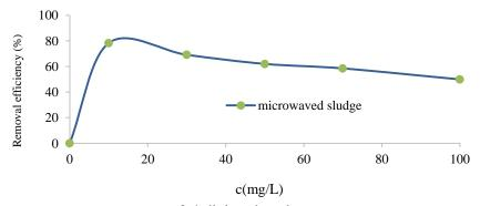
**Figure 4:** Effect of various concentrations of 2,4-dinitrophenol on adsorbent microwaved sludge (experimental condition; adsorbent dosage = 0.5 g 40 mL<sup>-1</sup>, optimal time and optimal pH)
