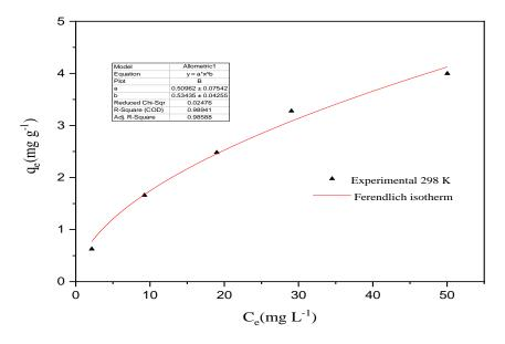
Figure 9: Non-linear diagram of Friendlich isotherm of the microwaved sludge
