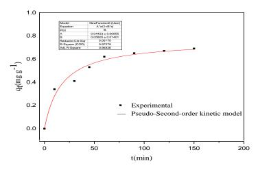
Figure 7: Non-linear pseudo-second-order diagram of the microwaved adsorbent
