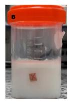
Figure 2: Change in the color of milk freshness label at 4 °C. A: Fresh milk; B: Spoiled milk.
