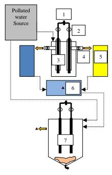
Figure 1: Scheme of the used electrolysis and electrocoagulation reactor
