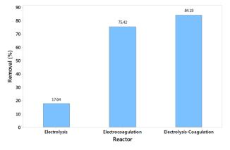
**Figure 4:** Comparison of removal efficiency in three studied reactors under optimum conditions (dye concentration; 10 mg/l, time; 60 min, voltage; 12)
