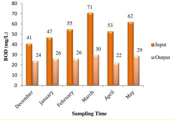
Figure 1: The trend of changes in BOD<sub>5</sub> in the input and output wastewater treatment plant
