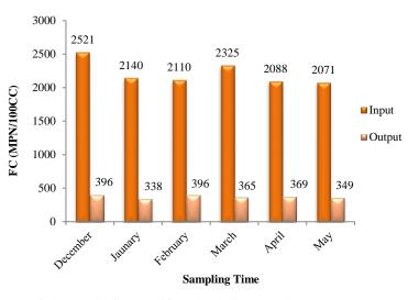
Figure 5: The trend of changes in fecal coliform in the input and output wastewater treatment plant
