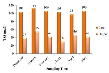
Figure 3: The trend of changes in TSS in the input and output wastewater treatment plant
