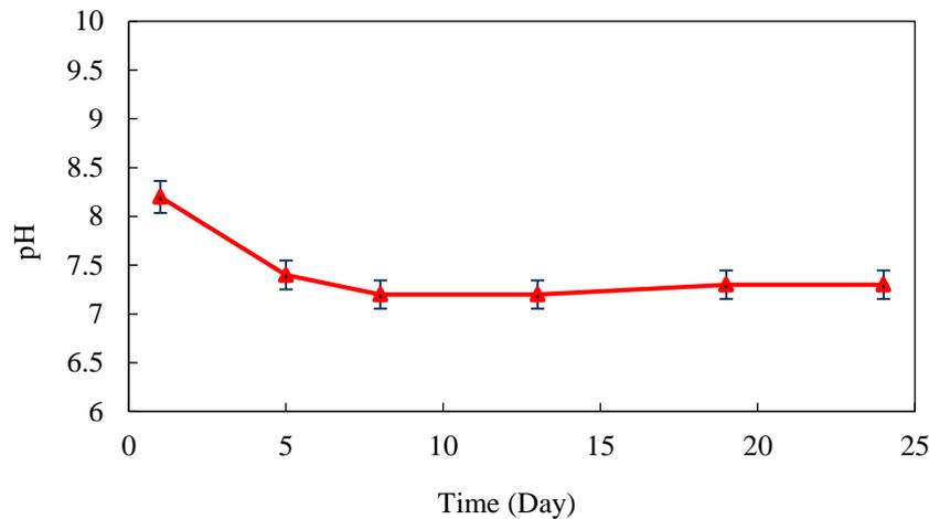
Figure 8: pH variations during the anaerobic digestion of wastewater sludge.
