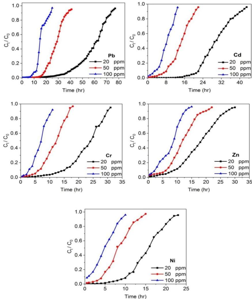
**Figure 5:** Effect of the influent concentration on the breakthrough time curve for Pb, Cd, Cr, Zn, and Ni
