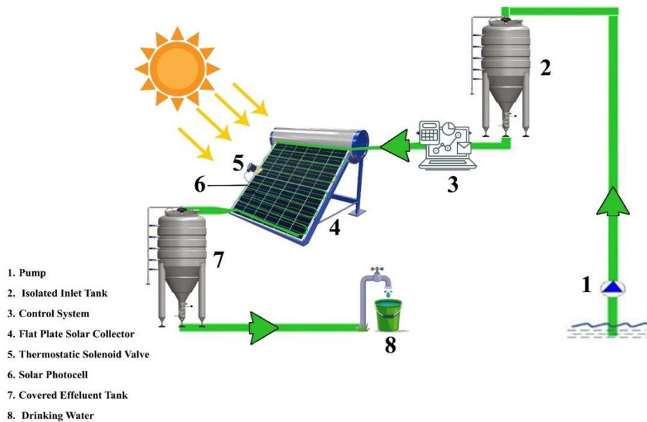
Figure 2: Schematic of the pilot
