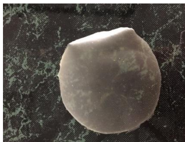
Figure 2: Edible film prepared by sourdough powder
