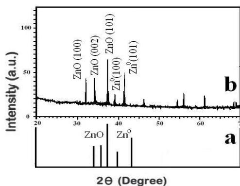
**Figure 2:** Standard Zn-ZnO powder diffraction pattern (a) and XRD pattern of nano nZ<sup>0</sup>-ZnO
