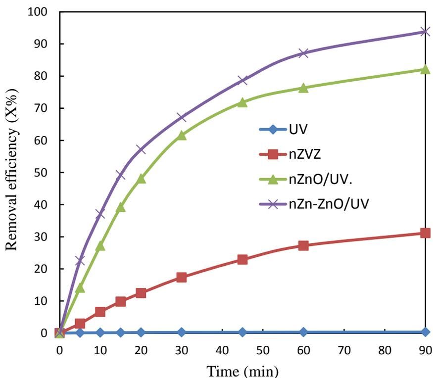
Figure 4: Removal efficiency (X%) of MO by the prepared redox nanocomposite in comparison with each of ZnO and Zn<sup>0</sup>.
