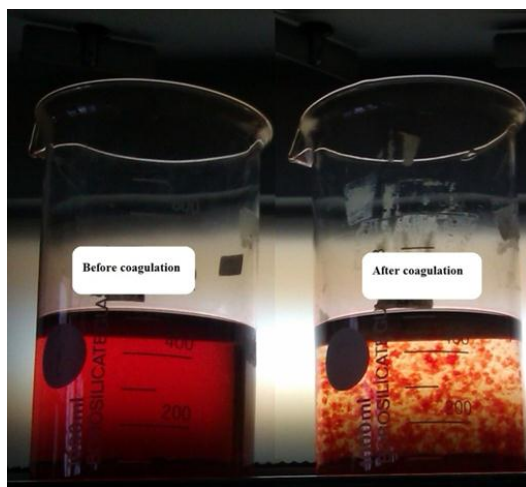
Figure 3: The image of dye solution before and after the coagulation (dye concentration: 50 mg/L, ferric chloride dose: 40 mg/L, pH 7)
