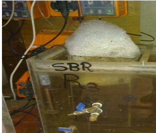
Figure 1: The SBR pilot with injection pump
