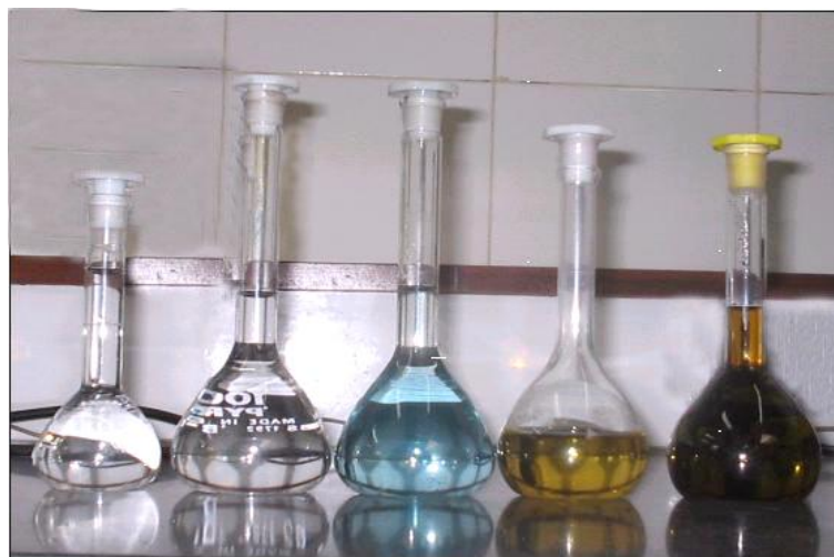
Figure 2: The effect of activated carbon dose on ADMI removal and removal efficiency (The dye concentration of 100 mg/L)
